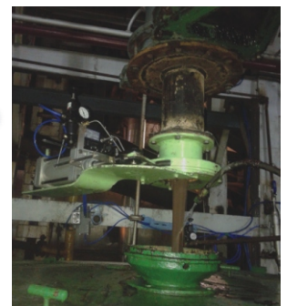
IRIS TYPE CONTROL VALVE INSTALLED ON CONTINUOUS CENTRIFUGAL MACHINE FOR AUTOMATIC MASSECUITE INTAKE WRT DRIVE LOAD
