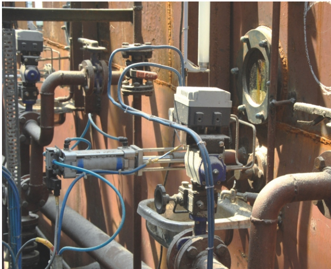
PICTURE OF YUTECH SELF CLEANING AUTO RETRACTABLE BRIX SENSOR INSTALLED ON CV PAN
